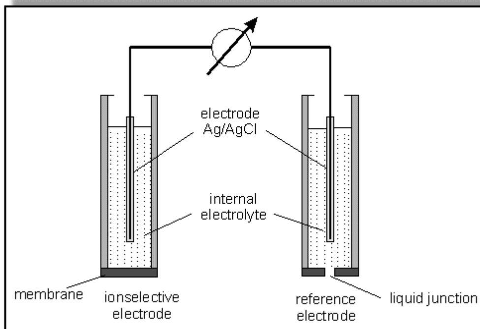
The sample above demonstrates the principles of electro-analytical measurements.
