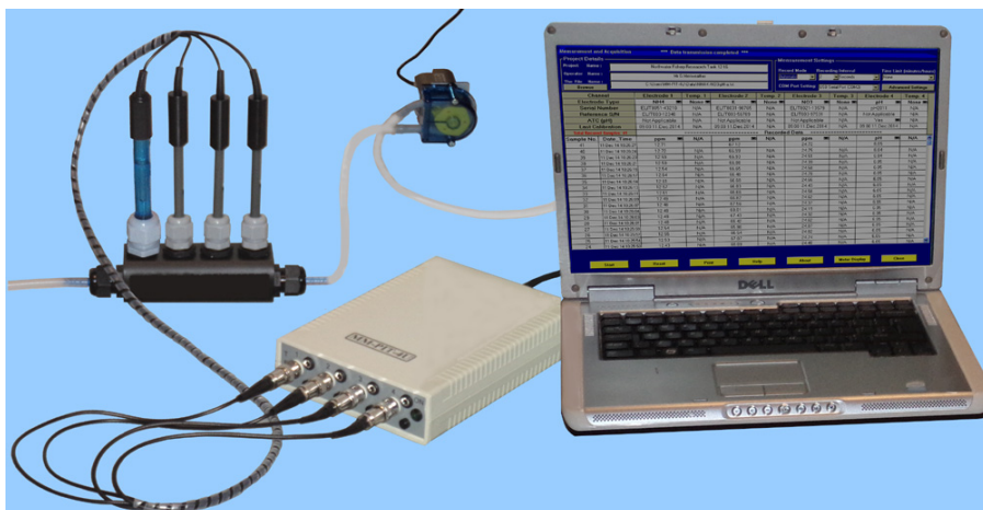
Flow-through Cell with 1xpH, 3x Ion selective Electrodes and 4-channel Monitor
